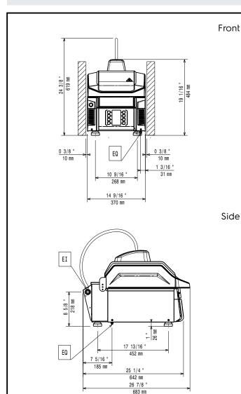
El = Electrical inlet (power) EO = Electrical Outlet
